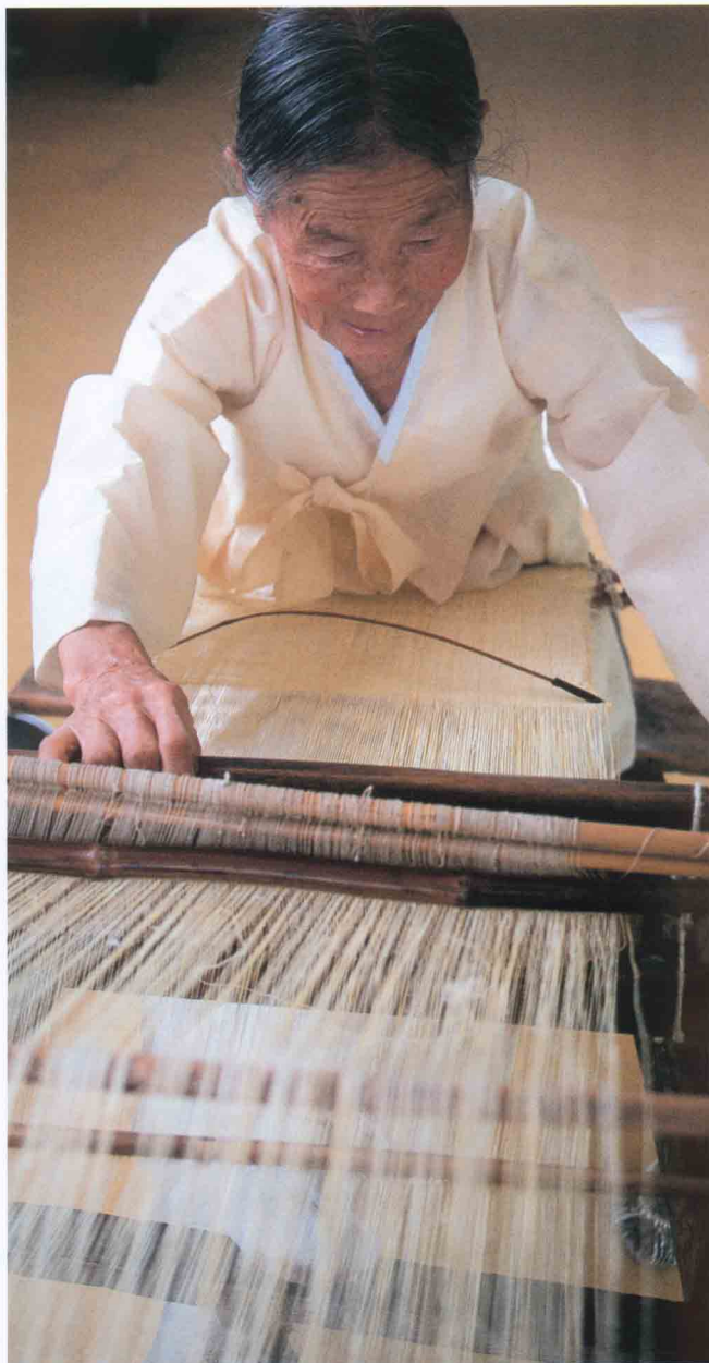
When the threads are ready, the warp is set up depending on the intended width of the cloth and the desired ply.
